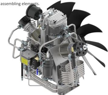
The bearings of the crankshaft have rollers, extremely robust and made in Europe which guarantee a long life of the compressor. An oil pump provides a constant lubrication of the inner workings of the block with oil cleaned of impurities by a filter and by a magnet which catches any metals present in the lubricating oil.
